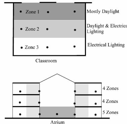
Daylighted zones of the selected space should be defined prior to the selection of the measurement points. These zones should be defined based on their distance from the window, (or atrium skylight), and based on the activity in the zone. Measurement points should represent typical illuminance in each daylighted zone. The number of daylighted zones and test points depend on the dimension of the space, and on the activity.
